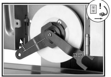
Figure 23. Removing wheel retaining nut.
